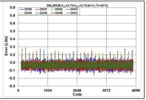
**FIGURE 2-83:** DNL Error vs. DAC Code,  $T = -40^{\circ}C$ ,  $V_{DD} = 2.7V$ .
