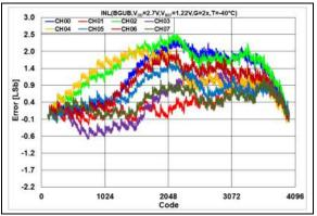
**FIGURE 2-41:** INL Error vs. DAC Code,  $T = -40^{\circ}$ C,  $V_{DD} = 2.7V$ .
