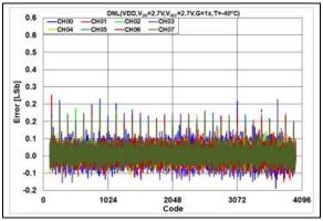
**FIGURE 2-26:** DNL Error vs. DAC Code,  $T = -40^{\circ}$ C,  $V_{DD} = 2.7$ V.
