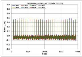
**FIGURE 2-88:** DNL Error vs. DAC Code, T = +125°C,  $V_{DD} = 5.5V$ .
