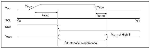
FIGURE 1-3: Power-on and Brown-out Reset Waveforms.
