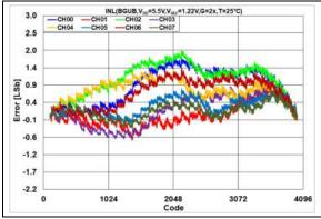
**FIGURE 2-39:** INL Error vs. DAC Code,  $T = +25^{\circ}C$ ,  $V_{DD} = 5.5V$ .
