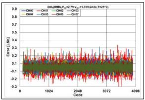
**FIGURE 2-126:** DNL Error vs. DAC Code,  $T = +25^{\circ}C$ ,  $V_{DD} = 2.7V$ .
