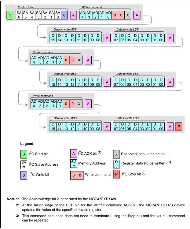
FIGURE 7-3: Continuous WRITE Commands (Volatile Memory Only).
