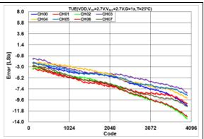
**FIGURE 2-15:** Total Unadjusted Error  $(V_{OUT})$  vs. DAC Code,  $T = +25^{\circ}C$ ,  $V_{DD} = 2.7V$ .
