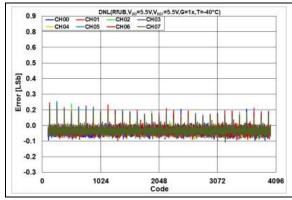
**FIGURE 2-80:** DNL Error vs. DAC Code,  $T = -40^{\circ}C$ ,  $V_{DD} = 5.5V$ .
