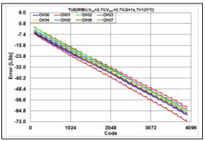
**FIGURE 2-97:** Total Unadjusted Error  $(V_{OUT})$  vs. DAC Code,  $T = +125^{\circ}C$ ,  $V_{DD} = 2.7V$ .
