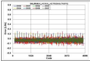
**FIGURE 2-87:** DNL Error vs. DAC Code,  $T = +25^{\circ}C$ ,  $V_{DD} = 5.5V$ .
