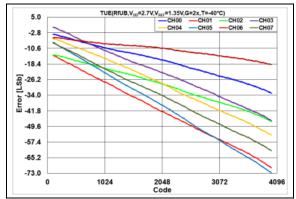
**FIGURE 2-65:** Total Unadjusted Error  $(V_{OUT})$  vs. DAC Code,  $T = -40^{\circ}C$ ,  $V_{DD} = 2.7V$ .
