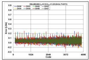
**FIGURE 2-48:** DNL Error vs. DAC Code,  $T = +25^{\circ}C V_{DD} = 5.5V.$
