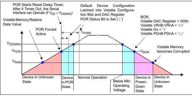
FIGURE 4-1: Power-On/Brown-Out Reset Operation.
