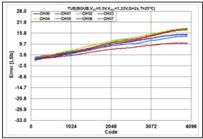
**FIGURE 2-30:** Total Unadjusted Error  $(V_{OUT})$  vs. DAC Code,  $T = +25^{\circ}C$ ,  $V_{DD} = 5.5V$ .
