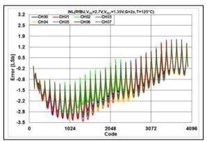
**FIGURE 2-115:** INL Error vs. DAC Code, T = +125°C,  $V_{DD} = 2.7V$ .
