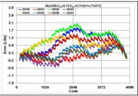
**FIGURE 2-21:** INL Error vs. DAC Code,  $T = +25^{\circ}C$ ,  $V_{DD} = 2.7V$ .
