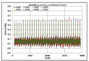
**FIGURE 2-127:** DNL Error vs. DAC Code, T = +125°C,  $V_{DD} = 2.7V$ .
