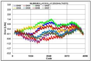
**FIGURE 2-45:** INL Error vs. DAC Code,  $T = +25^{\circ}C$ ,  $V_{DD} = 5.5V$ .
