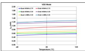
**FIGURE 2-1:** Average Device Supply Current vs. F<sub>SCL</sub> Frequency, Voltage and Temperature - Active Interface, VRnB:VRnA = 00, (V<sub>DD</sub> Mode).
