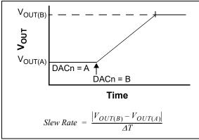
FIGURE 5-6: V<sub>OUT</sub> Pin Slew Rate.
