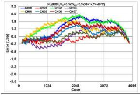
**FIGURE 2-104:** INL Error vs. DAC Code,  $T = -40^{\circ}C$ ,  $V_{DD} = 5.5V$ .
