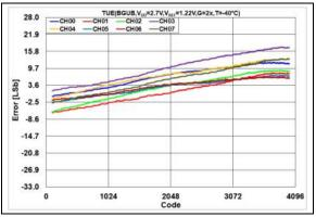
**FIGURE 2-32:** Total Unadjusted Error  $(V_{OUT})$  vs. DAC Code,  $T = -40^{\circ}C$ ,  $V_{DD} = 2.7V$ .
