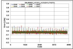
**FIGURE 2-81:** DNL Error vs. DAC Code,  $T = +25^{\circ}C$ ,  $V_{DD} = 5.5V$ .
