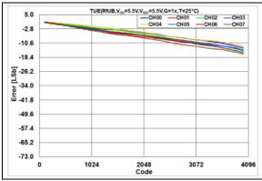
**FIGURE 2-57:** Total Unadjusted Error  $(V_{OUT})$  vs. DAC Code,  $T = +25^{\circ}C$ ,  $V_{DD} = 5.5V$ .
