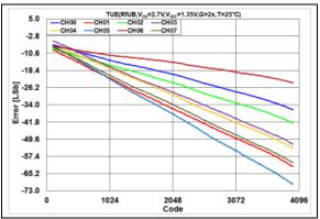
**FIGURE 2-66:** Total Unadjusted Error  $(V_{OUT})$  vs. DAC Code,  $T = +25^{\circ}C$ ,  $V_{DD} = 2.7V$ .
