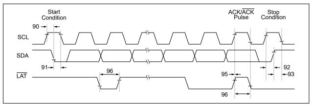
**FIGURE 1-5:**  $l^2C$  Bus Start/Stop Bits and LAT Timing Waveforms.
