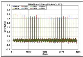
**FIGURE 2-25:** DNL Error vs. DAC Code, T = +125°C,  $V_{DD} = 5.5V$ .
