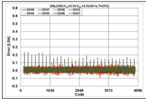
**FIGURE 2-24:** DNL Error vs. DAC Code,  $T = +25^{\circ}C$ ,  $V_{DD} = 5.5V$ .
