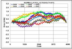
**FIGURE 2-110:** INL Error vs. DAC Code,  $T = -40^{\circ}C$ ,  $V_{DD} = 5.5V$ .
