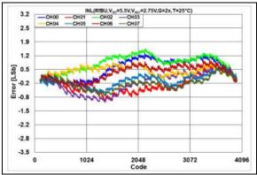
**FIGURE 2-111:** INL Error vs. DAC Code,  $T = +25^{\circ}C$ ,  $V_{DD} = 5.5V$ .
