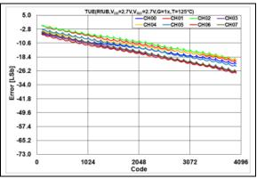
**FIGURE 2-61:** Total Unadjusted Error  $(V_{OUT})$  vs. DAC Code,  $T = +125^{\circ}C$ ,  $V_{DD} = 2.7V$ .
