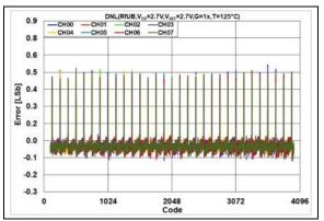
**FIGURE 2-85:** DNL Error vs. DAC Code,  $T = +125^{\circ}C, V_{DD} = 2.7V.$
