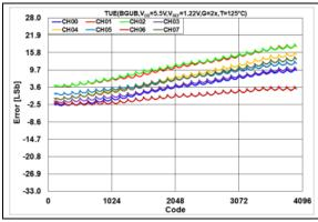
**FIGURE 2-31:** Total Unadjusted Error  $(V_{OUT})$  vs. DAC Code, T = +125°C,  $V_{DD} = 5.5V$ .
