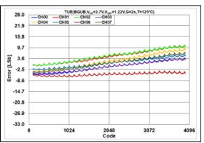
**FIGURE 2-34:** Total Unadjusted Error  $(V_{OUT})$  vs. DAC Code,  $T = +125^{\circ}$ C,  $V_{DD} = 2.7$ V.
