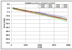
**FIGURE 2-92:** Total Unadjusted Error  $(V_{OUT})$  vs. DAC Code,  $T = -40^{\circ}C$ ,  $V_{DD} = 5.5V$ .
