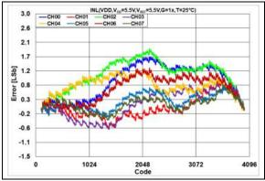
**FIGURE 2-18:** INL Error vs. DAC Code,  $T = +25^{\circ}C$ ,  $V_{DD} = 5.5V$ .
