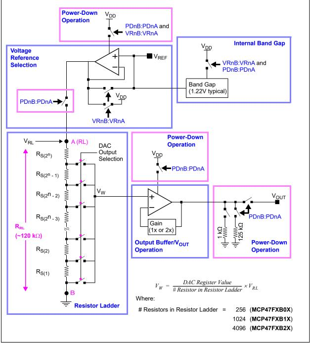
FIGURE 5-1: MCP47FXBX4/8 DAC Module Block Diagram.
