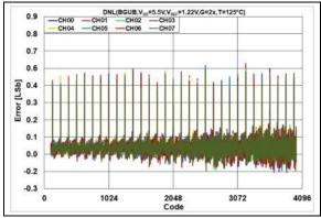
**FIGURE 2-49:** DNL Error vs. DAC Code,  $T = +125^{\circ}C$ ,  $V_{DD} = 5.5V$ .
