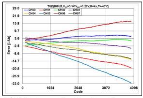
**FIGURE 2-35:** Total Unadjusted Error  $(V_{OUT})$  vs. DAC Code,  $T = -40^{\circ}C$ ,  $V_{DD} = 5.5V$ .
