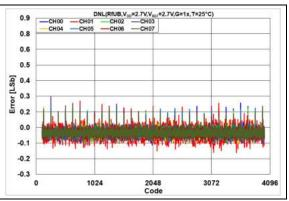
**FIGURE 2-84:** DNL Error vs. DAC Code,  $T = +25^{\circ}C$ ,  $V_{DD} = 2.7V$ .
