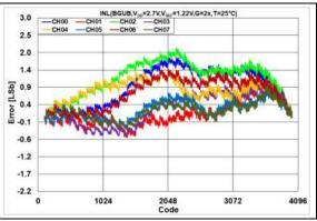
**FIGURE 2-42:** INL Error vs. DAC Code,  $T = +25^{\circ}C$ ,  $V_{DD} = 2.7V$ .
