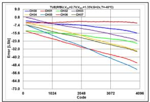
**FIGURE 2-101:** Total Unadjusted Error  $(V_{OUT})$  vs. DAC Code,  $T = -40^{\circ}C$ ,  $V_{DD} = 2.7V$ .
