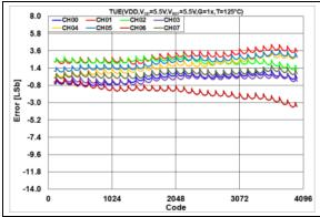
**FIGURE 2-13:** Total Unadjusted Error  $(V_{OUT})$  vs. DAC Code,  $T = +125^{\circ}C$ ,  $V_{DD} = 5.5V$ .
