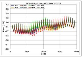
**FIGURE 2-73:** INL Error vs. DAC Code, T = +125°C,  $V_{DD} = 2.7V$ .
