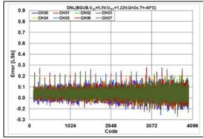
**FIGURE 2-47:** DNL Error vs. DAC Code,  $T = -40^{\circ}C$ ,  $V_{DD} = 5.5V$ .
