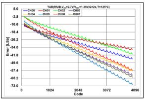
**FIGURE 2-67:** Total Unadjusted Error  $(V_{OUT})$  vs. DAC Code,  $T = +125^{\circ}C$ ,  $V_{DD} = 2.7V$ .
