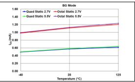
**FIGURE 2-5:** Average Device Supply Current - Inactive Interface (SCL =  $V_{IH}$  or  $V_{IL}$ ) vs. Voltage and Temperature, VRnB:VRnA = 01 (Band Gap Mode).
