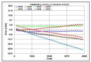
**FIGURE 2-37:** Total Unadjusted Error  $(V_{OUT})$  vs. DAC Code,  $T = +125^{\circ}C$ ,  $V_{DD} = 5.5V$ .
