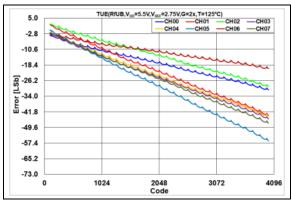
**FIGURE 2-64:** Total Unadjusted Error  $(V_{OUT})$  vs. DAC Code, T = +125°C,  $V_{DD} = 5.5V$ .
