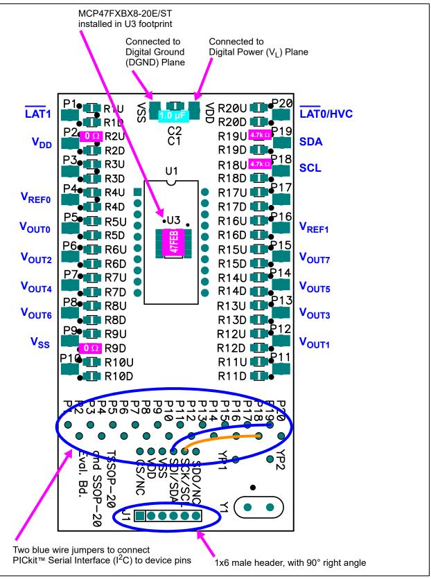
FIGURE 9-1: MCP47FXBX4/8 Evaluation Board Circuit Using TSSOP20EV.
