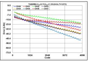
**FIGURE 2-103:** Total Unadjusted Error  $(V_{OUT})$  vs. DAC Code, T = +125°C,  $V_{DD} = 2.7V$ .
