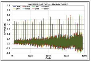
**FIGURE 2-52:** DNL Error vs. DAC Code,  $T = +125^{\circ}C, V_{DD} = 2.7V.$
