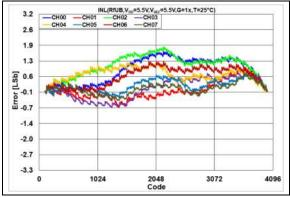
**FIGURE 2-69:** INL Error vs. DAC Code,  $T = +25^{\circ}C$ ,  $V_{DD} = 5.5V$ .
