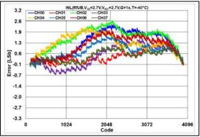
**FIGURE 2-71:** INL Error vs. DAC Code,  $T = -40^{\circ}$ C,  $V_{DD} = 2.7V$ .
