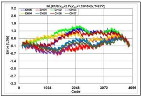
**FIGURE 2-78:** INL Error vs. DAC Code,  $T = +25^{\circ}C, V_{DD} = 2.7V.$
