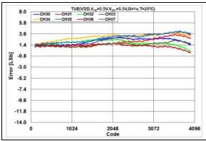
**FIGURE 2-12:** Total Unadjusted Error  $(V_{OUT})$  vs. DAC Code,  $T = +25^{\circ}C$ ,  $V_{DD} = 5.5V$ .
