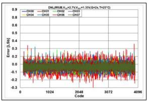
**FIGURE 2-90:** DNL Error vs. DAC Code,  $T = +25^{\circ}C$ ,  $V_{DD} = 2.7V$ .
