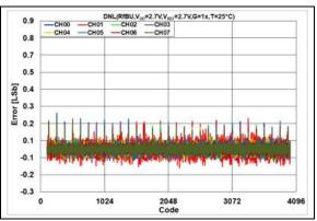
**FIGURE 2-120:** DNL Error vs. DAC Code,  $T = +25^{\circ}C, V_{DD} = 2.7V.$
