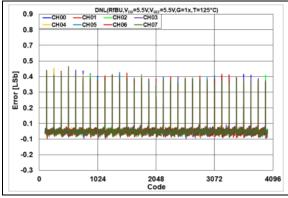
**FIGURE 2-118:** DNL Error vs. DAC Code,  $T = +125^{\circ}C, V_{DD} = 5.5V.$
