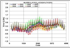
**FIGURE 2-19:** INL Error vs. DAC Code,  $T = +125^{\circ}C, V_{DD} = 5.5V.$
