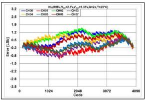
**FIGURE 2-114:** INL Error vs. DAC Code,  $T = +25^{\circ}C$ ,  $V_{DD} = 2.7V$ .
