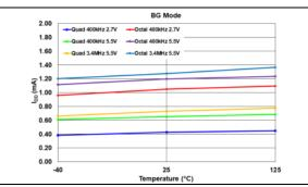
**FIGURE 2-2:** Average Device Supply Current vs.  $F_{SCL}$  Frequency, Voltage and Temperature - Active Interface, VRnB:VRnA = 01 (Band Gap Mode).
