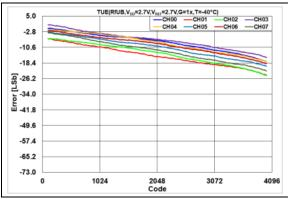
**FIGURE 2-59:** Total Unadjusted Error  $(V_{OUT})$  vs. DAC Code,  $T = -40^{\circ}C$ ,  $V_{DD} = 2.7V$ .
