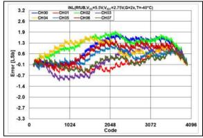
**FIGURE 2-74:** INL Error vs. DAC Code,  $T = -40^{\circ}$ C,  $V_{DD} = 5.5$ V.
