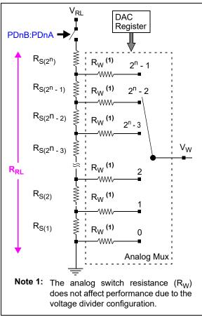
FIGURE 5-2: Resistor Ladder Model.
