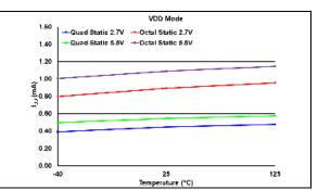
**FIGURE 2-4:** Average Device Supply Current - Inactive Interface (SCL =  $V_{IH}$  or  $V_{IL}$ ) vs. Voltage and Temperature, VRnB:VRnA = 00 ( $V_{DD}$  Mode).
