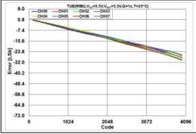
**FIGURE 2-93:** Total Unadjusted Error  $(V_{OUT})$  vs. DAC Code,  $T = +25^{\circ}C$ ,  $V_{DD} = 5.5V$ .
