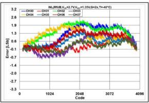
**FIGURE 2-77:** INL Error vs. DAC Code,  $T = -40^{\circ}$ C,  $V_{DD} = 2.7V$ .
