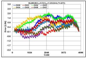
**FIGURE 2-44:** INL Error vs. DAC Code,  $T = -40^{\circ}C$ ,  $V_{DD} = 5.5V$ .
