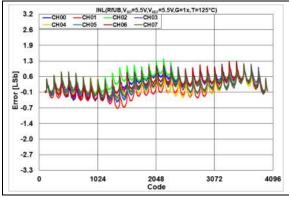
**FIGURE 2-70:** INL Error vs. DAC Code, T = +125°C,  $V_{DD} = 5.5V$ .
