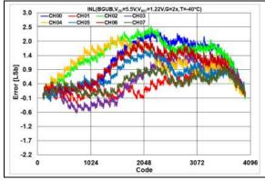
**FIGURE 2-38:** INL Error vs. DAC Code,  $T = -40^{\circ}C$ ,  $V_{DD} = 5.5V$ .
