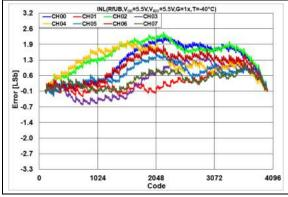
**FIGURE 2-68:** INL Error vs. DAC Code,  $T = -40^{\circ}C$ ,  $V_{DD} = 5.5V$ .
