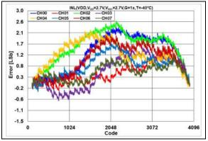
**FIGURE 2-20:** INL Error vs. DAC Code,  $T = -40^{\circ}$ C,  $V_{DD} = 2.7V$ .
