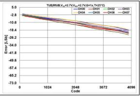
**FIGURE 2-60:** Total Unadjusted Error  $(V_{OUT})$  vs. DAC Code,  $T = +25^{\circ}C$ ,  $V_{DD} = 2.7V$ .
