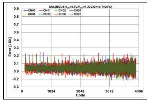
**FIGURE 2-54:** DNL Error vs. DAC Code,  $T = +25^{\circ}$ C,  $V_{DD} = 5.5V$ .
