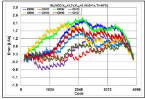
**FIGURE 2-17:** INL Error vs. DAC Code,  $T = 40^{\circ}$ C,  $V_{DD} = 5.5V$ .
