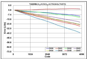
**FIGURE 2-99:** Total Unadjusted Error  $(V_{OUT})$  vs. DAC Code,  $T = +25^{\circ}C, V_{DD} = 5.5V.$
