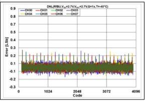
**FIGURE 2-119:** DNL Error vs. DAC Code,  $T = -40^{\circ}C$ ,  $V_{DD} = 2.7V$ .
