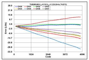
**FIGURE 2-36:** Total Unadjusted Error  $(V_{OUT})$  vs. DAC Code,  $T = +25^{\circ}C$ ,  $V_{DD} = 5.5V$ .
