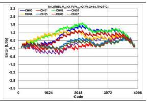
**FIGURE 2-108:** INL Error vs. DAC Code,  $T = +25^{\circ}C$ ,  $V_{DD} = 2.7V$ .
