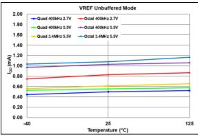
FIGURE 2-7:Average Device SupplyCurrent vs.  $F_{SCL}$  Frequency, Voltage andTemperature - Active Interface,VRnB:VRnA = 10 (V<sub>REF</sub> Unbuffered Mode).
