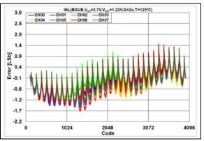
**FIGURE 2-43:** INL Error vs. DAC Code, T = +125°C,  $V_{DD} = 2.7V$ .
