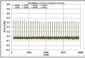
**FIGURE 2-82:** DNL Error vs. DAC Code,  $T = +125^{\circ}C, V_{DD} = 5.5V.$
