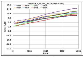
**FIGURE 2-29:** Total Unadjusted Error  $(V_{OUT})$  vs. DAC Code, T = -40°C,  $V_{DD} = 5.5V$ .
