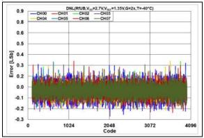
**FIGURE 2-89:** DNL Error vs. DAC Code,  $T = -40^{\circ}$ C,  $V_{DD} = 2.7$ V.
