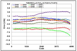
**FIGURE 2-14:** Total Unadjusted Error  $(V_{OUT})$  vs. DAC Code,  $T = -40^{\circ}C$ ,  $V_{DD} = 2.7V$ .
