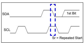
FIGURE B-5: REPEAT START CONDITION WAVEFORM.
