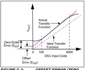
FIGURE C-2: OFFSET ERROR (ZERO GAIN ERROR).
