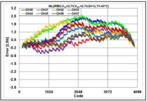
**FIGURE 2-107:** INL Error vs. DAC Code,  $T = -40^{\circ}$ C,  $V_{DD} = 2.7V$ .
