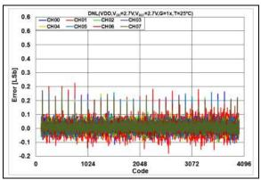
**FIGURE 2-27:** DNL Error vs. DAC Code,  $T = +25^{\circ}C$ ,  $V_{DD} = 2.7V$ .
