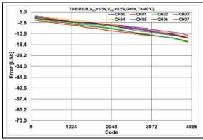
**FIGURE 2-56:** Total Unadjusted Error  $(V_{OUT})$  vs. DAC Code,  $T = -40^{\circ}C$ ,  $V_{DD} = 5.5V$ .
