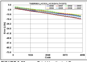
**FIGURE 2-58:** Total Unadjusted Error  $(V_{OUT})$  vs. DAC Code,  $T = +125^{\circ}$ C,  $V_{DD} = 5.5$ V.
