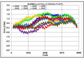
**FIGURE 2-113:** INL Error vs. DAC Code,  $T = -40^{\circ}$ C,  $V_{DD} = 2.7$ V.
