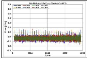
**FIGURE 2-86:** DNL Error vs. DAC Code,  $T = -40^{\circ}C$ ,  $V_{DD} = 5.5V$ .
