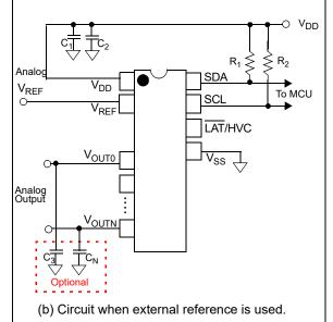
$R_1$  and  $R_2$  are I<sup>2</sup>C pull-up resistors:
