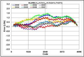
**FIGURE 2-105:** INL Error vs. DAC Code,  $T = +25^{\circ}C$ ,  $V_{DD} = 5.5V$ .
