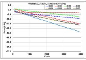
**FIGURE 2-100:** Total Unadjusted Error  $(V_{OUT})$  vs. DAC Code, T = +125°C,  $V_{DD} = 5.5V$ .
