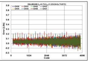
**FIGURE 2-51:** DNL Error vs. DAC Code,  $T = +25^{\circ}C V_{DD} = 2.7V.$
