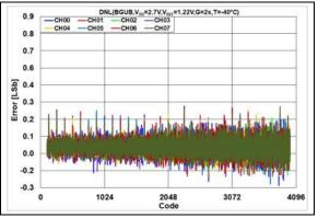
**FIGURE 2-50:** DNL Error vs. DAC Code,  $T = -40^{\circ}C$ ,  $V_{DD} = 2.7V$ .
