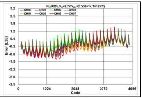
**FIGURE 2-109:** INL Error vs. DAC Code, T = +125°C,  $V_{DD} = 2.7V$ .
