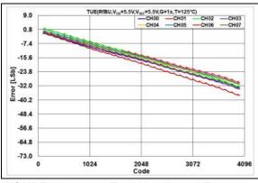
**FIGURE 2-94:** Total Unadjusted Error  $(V_{OUT})$  vs. DAC Code, T = +125°C,  $V_{DD} = 5.5V$ .
