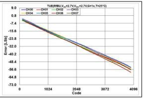
**FIGURE 2-96:** Total Unadjusted Error  $(V_{OUT})$  vs. DAC Code,  $T = +25^{\circ}C$ ,  $V_{DD} = 2.7V$ .
