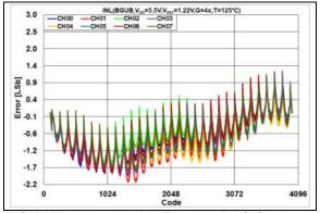
**FIGURE 2-46:** INL Error vs. DAC Code,  $T = +125^{\circ}C$ ,  $V_{DD} = 5.5V$ .
