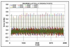
**FIGURE 2-91:** DNL Error vs. DAC Code,  $T = +125^{\circ}C, V_{DD} = 2.7V.$
