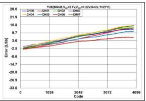
**FIGURE 2-33:** Total Unadjusted Error  $(V_{OUT})$  vs. DAC Code,  $T = +25^{\circ}C$ ,  $V_{DD} = 2.7V$ .
