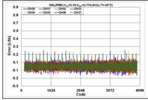
**FIGURE 2-122:** DNL Error vs. DAC Code,  $T = -40^{\circ}C$ ,  $V_{DD} = 5.5V$ .
