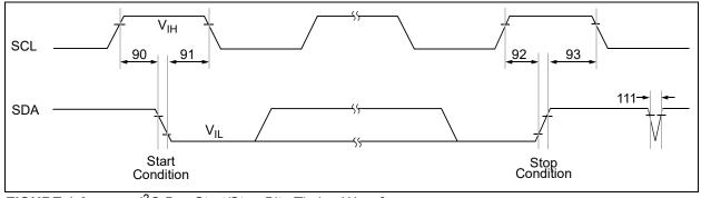
**FIGURE 1-6:** I<sup>2</sup>C Bus Start/Stop Bits Timing Waveforms.
