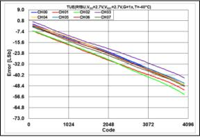
**FIGURE 2-95:** Total Unadjusted Error  $(V_{OUT})$  vs. DAC Code,  $T = -40^{\circ}C$ ,  $V_{DD} = 2.7V$ .
