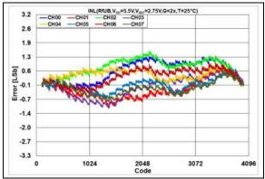
**FIGURE 2-75:** INL Error vs. DAC Code,  $T = +25^{\circ}C$ ,  $V_{DD} = 5.5V$ .
