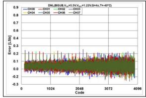
**FIGURE 2-53:** DNL Error vs. DAC Code,  $T = -40^{\circ}C$ ,  $V_{DD} = 5.5V$ .
