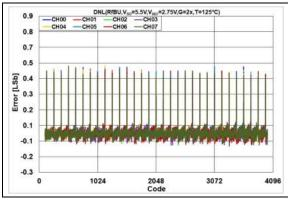
**FIGURE 2-124:** DNL Error vs. DAC Code, T = +125°C,  $V_{DD} = 5.5V$ .
