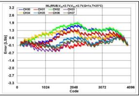
**FIGURE 2-72:** INL Error vs. DAC Code,  $T = +25^{\circ}C$ ,  $V_{DD} = 2.7V$ .
