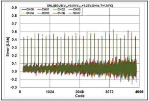
**FIGURE 2-55:** DNL Error vs. DAC Code,  $T = +125^{\circ}C$ ,  $V_{DD} = 5.5V$ .
