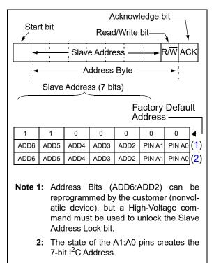
**FIGURE 6-2:** Slave Address Bits in the I<sup>2</sup>C Control Byte.
