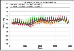
**FIGURE 2-106:** INL Error vs. DAC Code, T = +125°C,  $V_{DD} = 5.5V$ .
