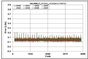
**FIGURE 2-117:** DNL Error vs. DAC Code,  $T = +25^{\circ}$ C,  $V_{DD} = 5.5V$ .
