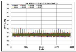
**FIGURE 2-116:** DNL Error vs. DAC Code,  $T = -40^{\circ}C$ ,  $V_{DD} = 5.5V$ .
