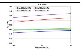
FIGURE 2-6:Average Device SupplyCurrent - Inactive Interface (SCL =  $V_{IH}$  or  $V_{IL}$ ) vs.Voltage and Temperature, VRnB:VRnA = 11( $V_{REF}$  Buffered Mode).
